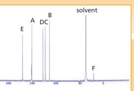
4 hours polarisation, single scan Limit of detection S/N of 10 on the smallest peak F
