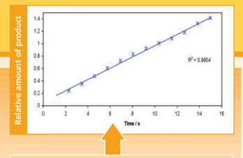
From ratio of peak integral, at 172.3ppm (reaction:control) kinetic rates can be determined<sup>1</sup>
