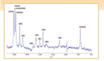
NMR of complex mixtures can be difficult due to low sensitivity and spectral crowding for <sup>1</sup>H spectra. Conventional <sup>13</sup>C NMR offers greater chemical shift dispersion but with lower sensitivity.
