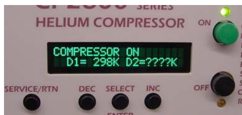
Figure 7-4: Display panel of the compressor package at start up
