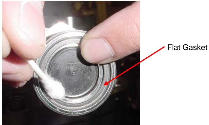
Figure B-2: Cleaning the male Aeroquip®
