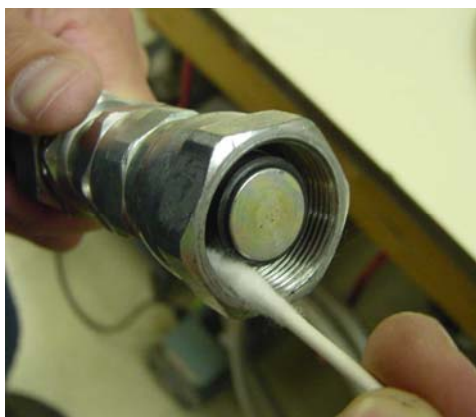
Figure B-1: Cleaning the female Aeroquip
