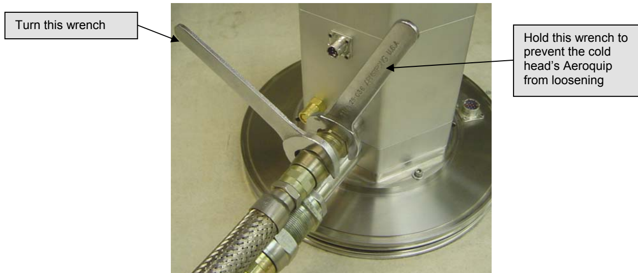
Figure 7-2: Disconnecting flex lines from a cold head
