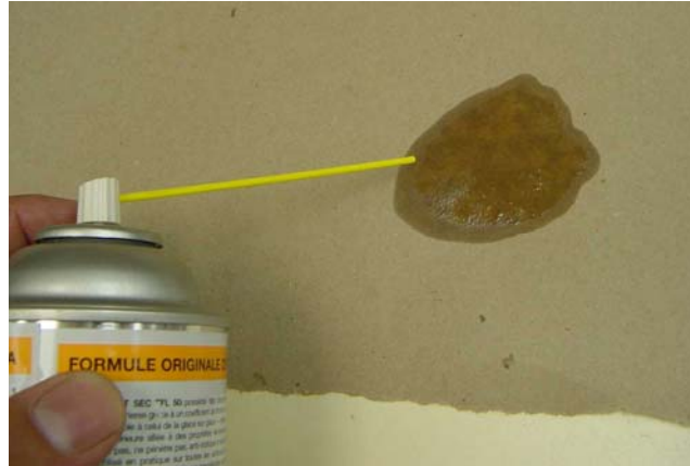
Figure B-4: Typical amount of lubricant
