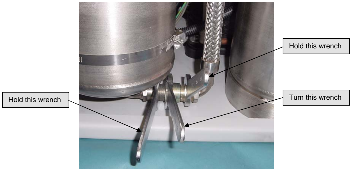
Figure 10: Disconnecting the adsorber.
