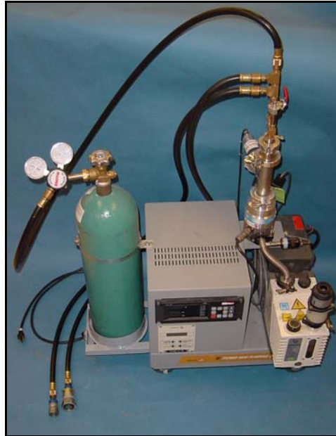
Figure 10: Helium recharging assembly
