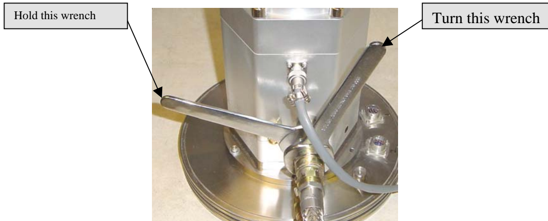
Figure 9: Disconnecting Aeroquips® from the cold head
