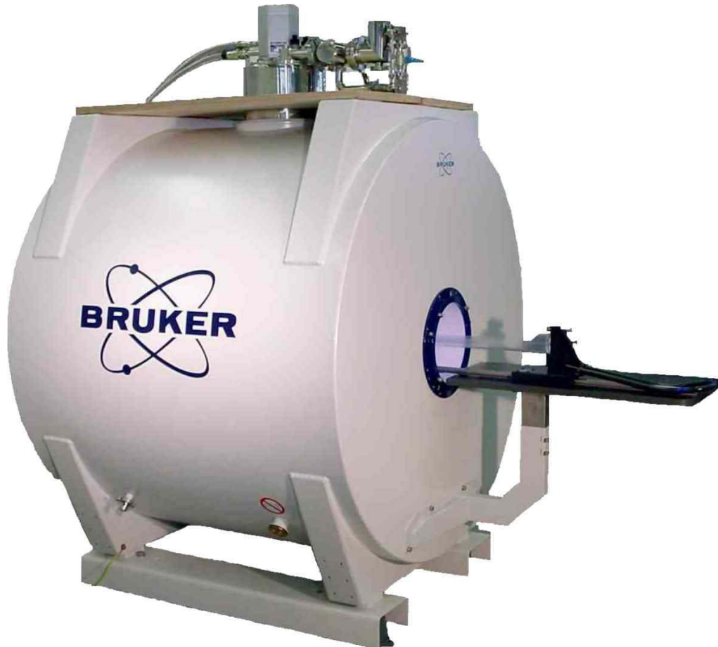
Figure 11: View of a Bruker USR magnet system
