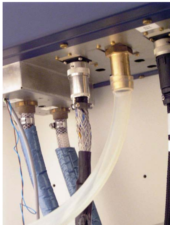
Figure 17: Anesthesia gas outlet is connected with a silicone tube. Filter box on rear side of the magnet (solution without Faraday cage)
