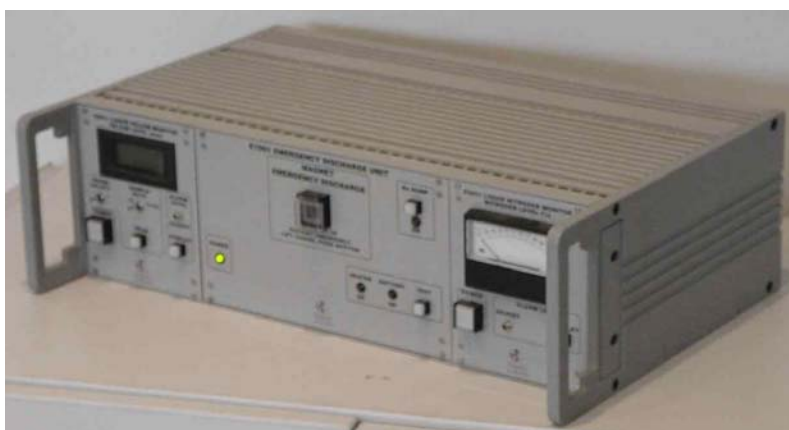
Figure 31: Emergency Discharge (Magnet Run-down Unit for a Magnex AS Magnet)
