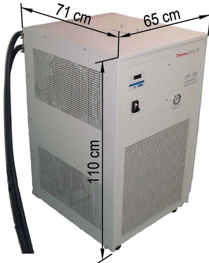
Figure 29: View of the Thermo NESLAB CFT-300 water chiller system
